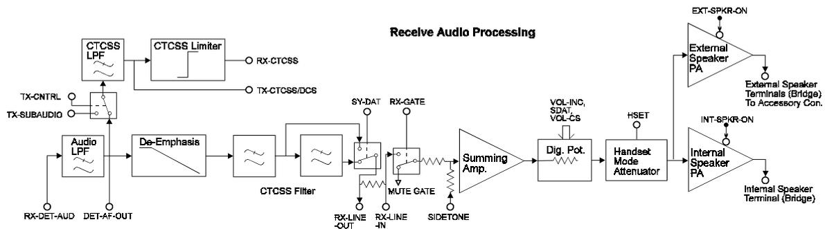
**Note:** All switches are drawn in the position where the relevant signal is 0V.
