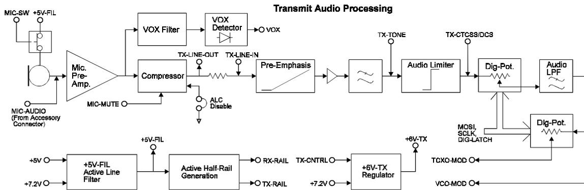
**Note:** All switches are drawn in the position where the relevant control signal is 0V.
