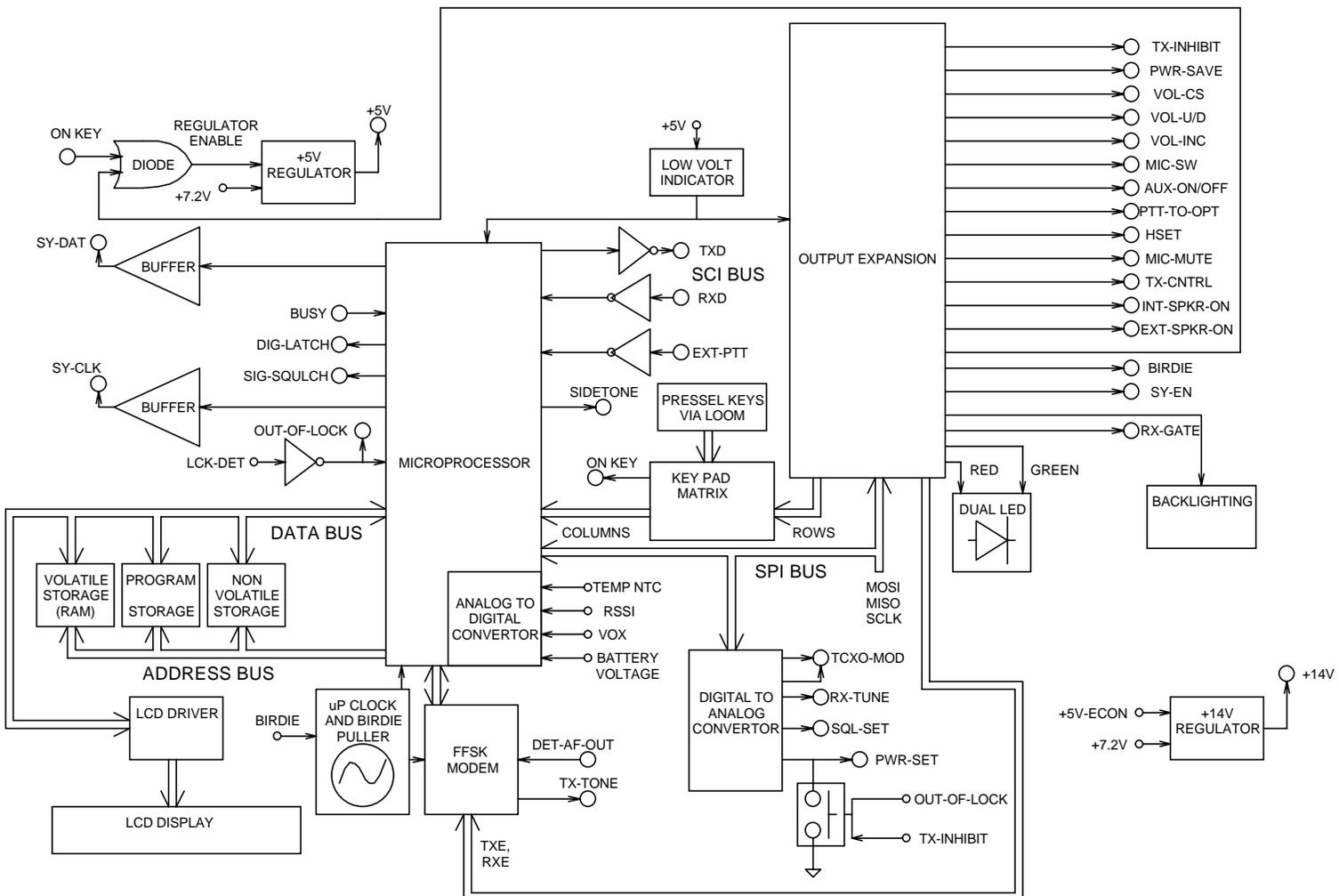
Figure 2.3 T3020, T3030, T3035 & T3040 Control PCB Block Diagram
